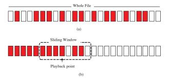
Fig. 4. Buffer snapshots of BitTorrent (a) and CoolStreaming (b), where shaded segments are available in the buffer.
