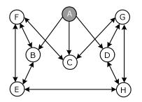
Fig. 3. An illustration of partnerships in the pull-based peerto-peer streaming system with A being the source.
