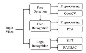
Figure 2: Block diagram of the face and logo recognition processing
