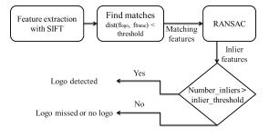
Figure 4: Illustration of the logo detection algorithm
