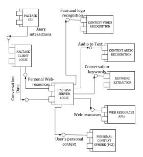
Figure 1: Component architecture of the integrated components
