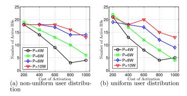
Figure 5: Number of active BSs versus transmission power and activation cost.
