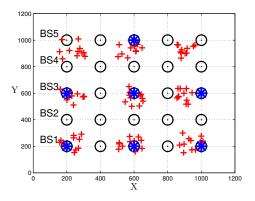
Figure 2: Snapshot of activated base stations (\*\*) in a network with non-uniform user distribution .
